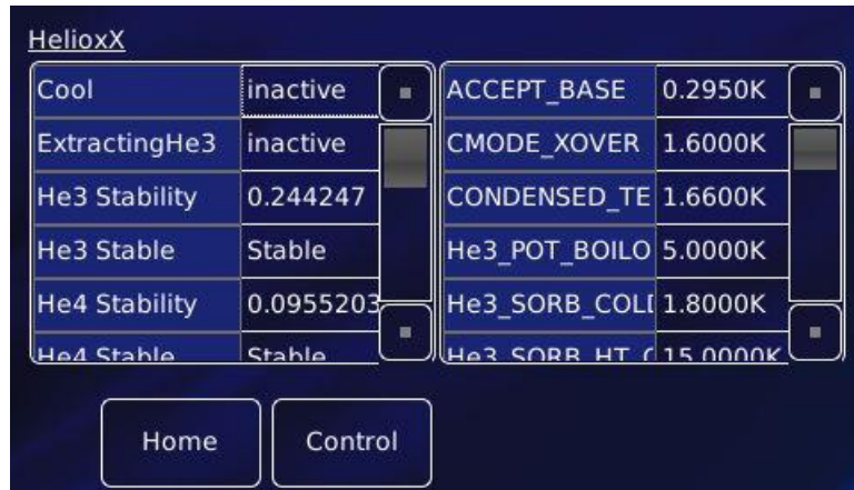
Figure 5-6: MercuryTC Heliox Controller settings screen.
