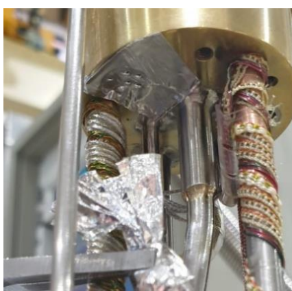
Figure 5-1: Aluminium foil tape (with pierced holes) covering the line-of-sight port. NRC2 foil (shown underneath) is added inside the port before it is taped over.
